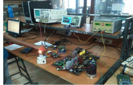
Figure 9: Experimental set-up of the solar inverter module
